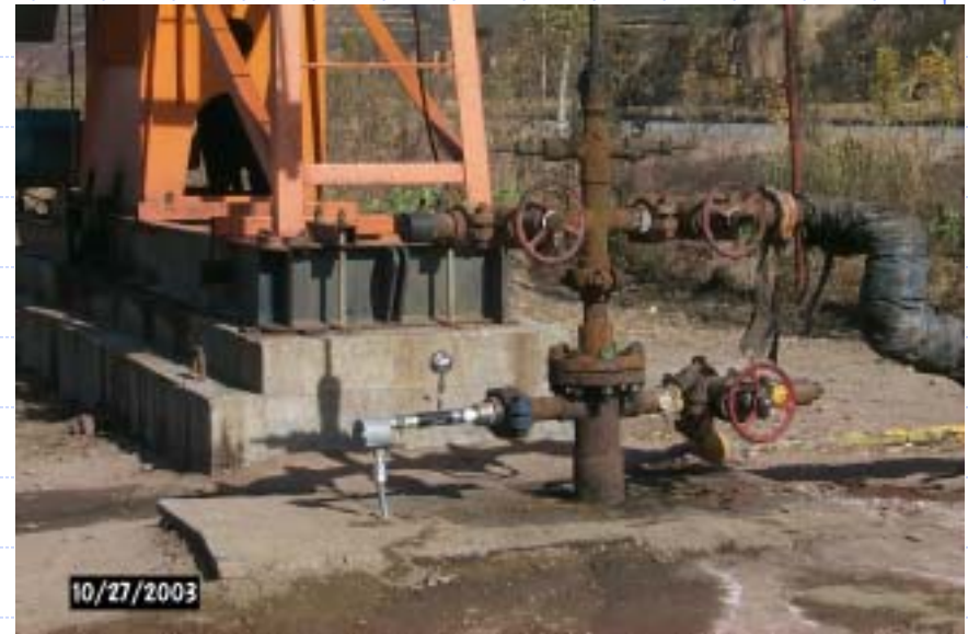
Well head with Downhole gauge packoff
